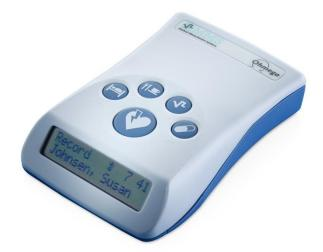
There is a small chance of battery failure, however even if the screen goes dark and will not light up, the device will probably still be recording – please continue to use it. Do not try to change the batteries.
